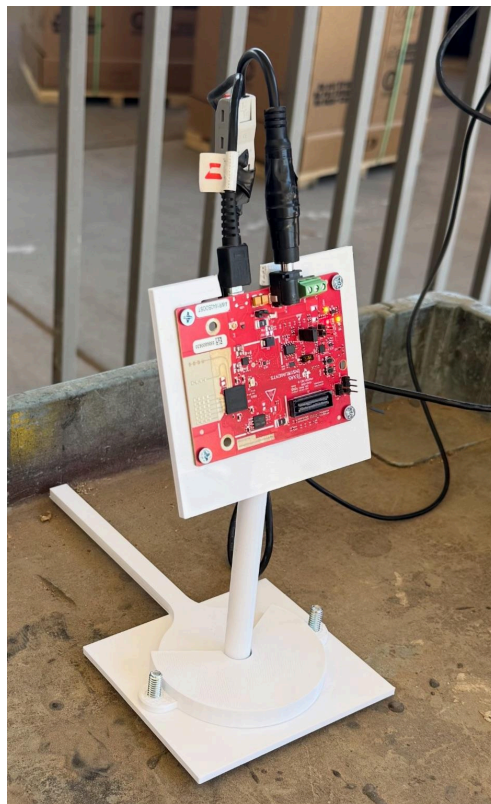
Figure 17. Radar mount prototype
