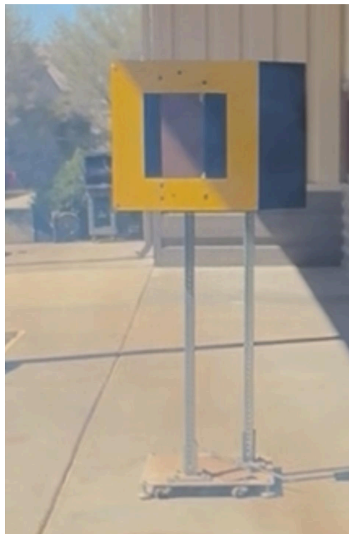
Figure 14. Modified sign face with bisected face prototype
