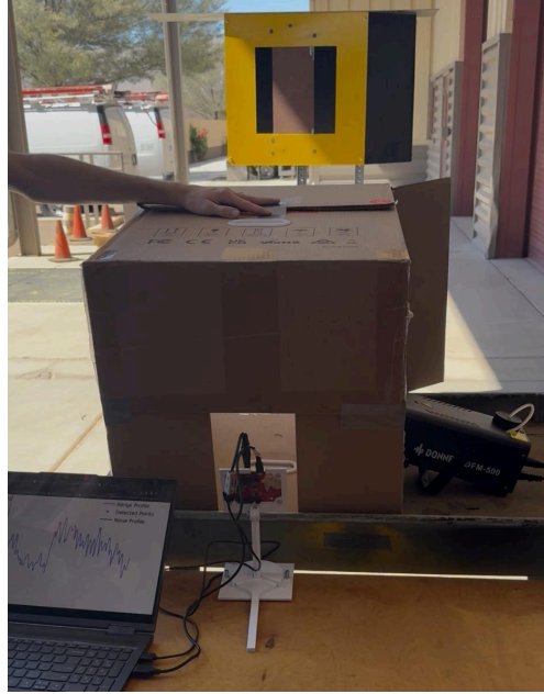
Figure 20. Test setup for fog testing using a box for containment
