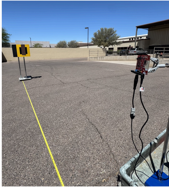
Figure 19. Test setup for angle testing at 30 degrees
